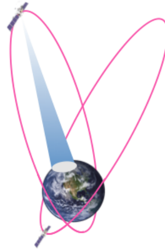
Figure 6: A dedicated satellite constellation using Highly Elliptical Orbit (HEO) would take care of GNSS augmentation data broadcast as well as many other communications needs in the Arctic (A. B. O. Jensen 2010). Courtesy of the Canadian Space Agency (CSA).
